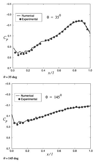
Fig. 14 Comparison of surface pressure coefficient in the longitudinal direction between the computational and experimental data at different azimuthal angles.
