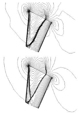
Fig. 9 Pressure contours on the initial and level 3 adaptive grid for ONERA M6 wing (M = 0.84 and  $\alpha$  = 3.06).
