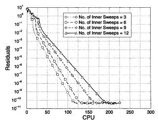
Fig. 4  $\,$  Effect of number of inner iterations on the convergence rate of BLU-SGS.
