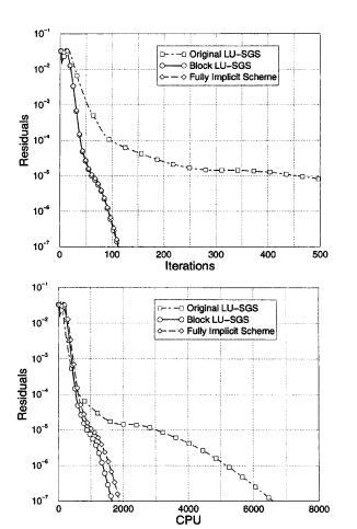
Fig. 12 Convergence histories in terms of iterations and CPU seconds for supersonic turbulent flow over the analytical forebody.
