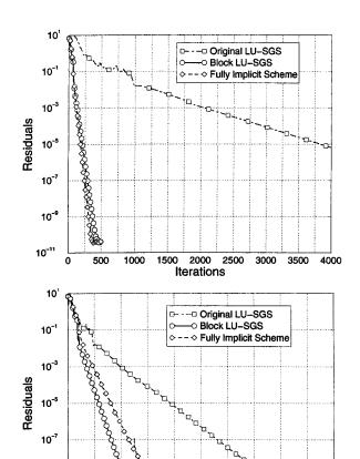
Fig. 5 Comparison of convergence characteristics between LU-SGS, BLU-SGS, and FIS in terms of number of iterations and CPU seconds on a Pentium III 450.
