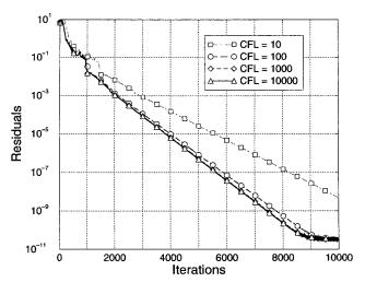
Fig. 2 Effect of CFL number on the convergence rate of LU-SGS.
