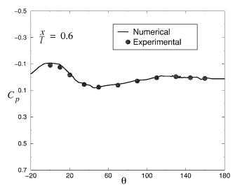
Fig. 13 Comparison of surface pressure coefficient in the azimuthal direction between computational and experimental data at different axial locations.
