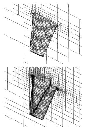
Fig. 7 Initial and level 3 anisotropic adaptive Cartesian grid for the ONERA M6 wing.
