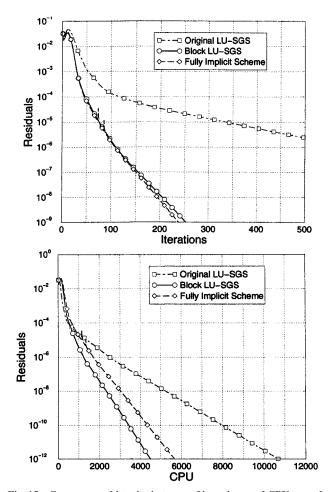
Fig. 15 Convergence histories in terms of iterations and CPU seconds for supersonic laminar flow over the analytical forebody.
