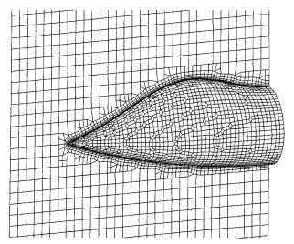
Fig. 11 Viscous Cartesian computational grid around the analytical forebody.
