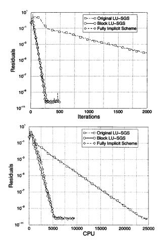
Fig. 8 Comparison of convergence characteristics between LU-SGS, BLU-SGS, and FIS in terms of number of iterations and CPU seconds for transonic flow over ONERA M6 wing.
