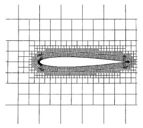
Fig. 1  $\,$  Adaptive Cartesian/quad unstructured grid around the NACA 0012 airfoil.
