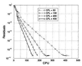
Fig. 3 Effect of CFL number on the convergence rate of BLU-SGS.
